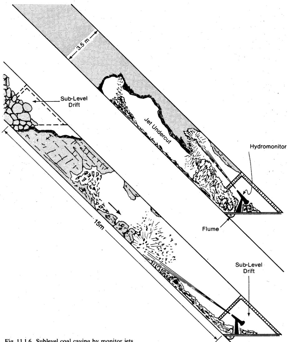
Fig. 11.1.6. Sublevel coal caving by monitor jets.
