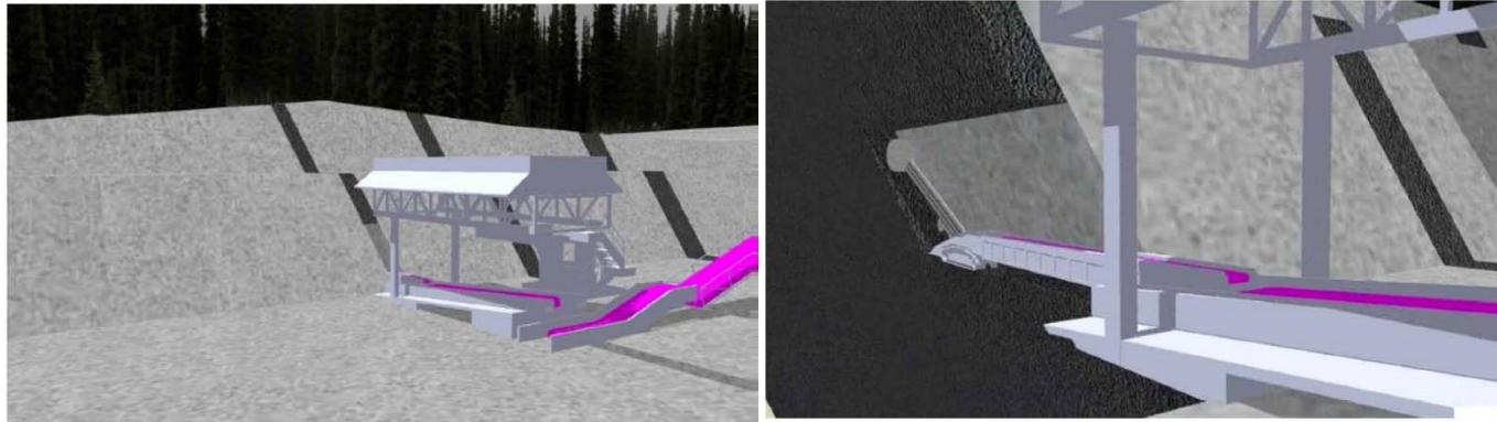
1. Launch vehicle positioned on mine bench in front of steeply dipping seam exposed in highwall
