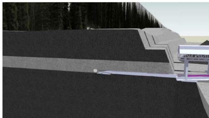
3. Profile of ADDCAR unit retreating from mined entry. Note pillar of coal above mined out entry.
